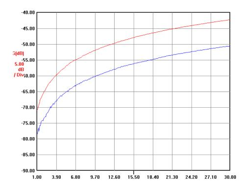
Top Curve: Receiver to Transmitter isolation when on Receive. (The transmitter is 50ohms above ground in the dummy load.) Bottom Curve: Receiver to Transmitter isolation when on Transmit. (The receiver is grounded.)
