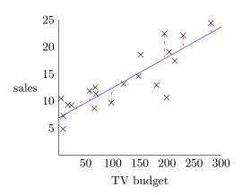
Each  $\times$  represents a data point. Also represented on the scatterplot is the (least squares) line of best fit: this is the unique line y = mx + b that minimises the average of the sum of the squares of the lengths of the red dashed lines. This quantity is known as the root mean square error (RMSE):
