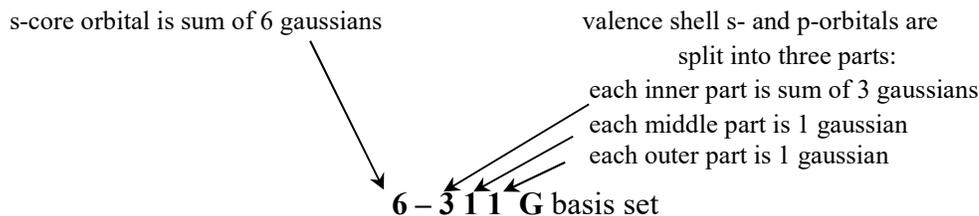
Figure 25.5.4: A 6-311G Gaussian basis set uses a triply split valence shell.
