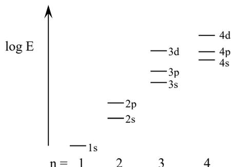
Figure 25.4.4: Relative orbital energies for K ( $Z = 19$ ) and Ca ( $Z = 20$ ). The log energy axis allows the core and valence orbital energies to be plotted on the same convenient scale.
