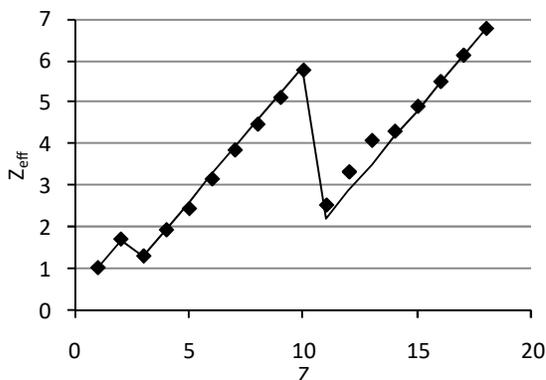
Figure 25.5.1: The  $Z_{\text{eff}}$  approximated using Slater's rules versus the SCF-optimized values from Table 25.5.1, for the highest energy sub-shell.
