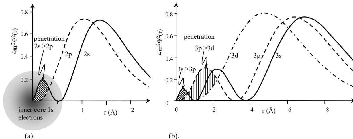
Figure 25.4.3: Low  $\ell$  orbitals penetrate closer to the nucleus and feel a greater effective nuclear charge than high  $\ell$  orbitals. (a). The 1s-electrons shield the 2s and 2p electrons from the full nuclear charge. (b). The 1s, 2s, and 2p-electrons shield the 3s, 3p, and 3d electrons from the full nuclear charge. Because of decreasing penetration,  $Z_{\text{eff}}(3s) > Z_{\text{eff}}(3p) > Z_{\text{eff}}(3d)$ .
