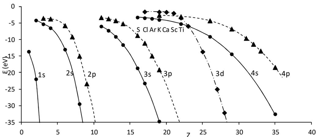
Figure 25.4.2: Atomic orbital energies from self-consistent field calculations.<sup>2</sup> Plotting symbols: s-orbitals  $\bullet$ —, p-orbitals  $\blacktriangle$ - - -, 3d-orbital  $\blacklozenge$ -·-·.
