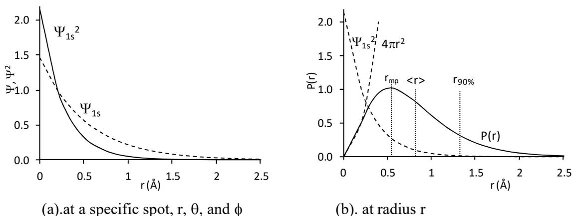
Figure 25.1.2: (a). The probability of finding the electron in a 1s-orbital in a narrow range around  $(r, \theta, \phi)$  is proportional to  $\Psi^2$ . (b). The probability of finding an electron at a radius  $r$ , irrespective of angles, is given by  $P(r) dr = \Psi^2 4\pi r^2 dr$ .
