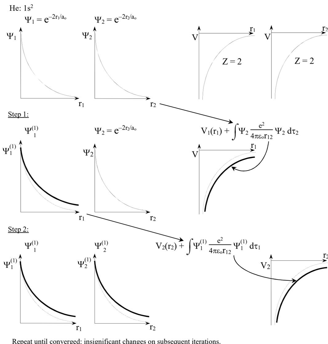
Figure 25.4.1: Self-consistent field calculations are iterative. The expectation value of the electron-electron repulsion is averaged over the coordinates of the opposite electron.
