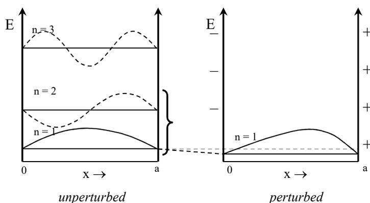
Figure 25.3.3: The first order correction mixes excited state character into the unperturbed wave function. For a particle in a box in an external electric field, mixing small amounts of the  $n = 2$  wave function into the ground state skews the electron distribution in response to the perturbation. Low energy excited states contribute more to the correction than high energy excited states.
