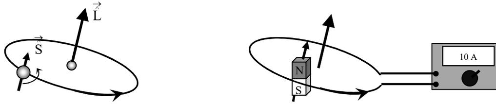
Figure 25.6.4: The magnetic field generated by the orbital motion of the electron and the intrinsic magnetic moment of the electron interact like a bar magnet in the magnetic field created by electrical current in a loop of wire.
