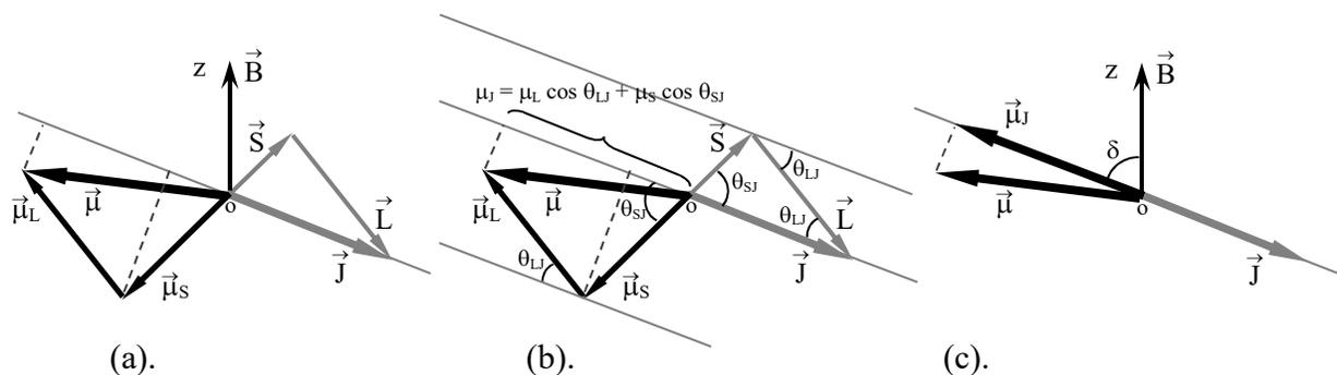
Figure 25.7.1: (a). The orbital and spin angular momenta add vectorially. The orbital and spin magnetic moments also add vectorially. (b). The Law of Cosines determines the angles relative to the total angular momentum. The effective magnetic moment,  $\vec{\mu}_J$ , is collinear with  $\vec{J}$ . (c). The interaction with the external magnetic field is:  $\Delta E = -\vec{\mu}_J \cdot \vec{B} = -\mu_J B \cos \delta$ .
