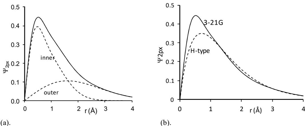
Figure 25.5.3: (a). The 3-21G basis set has a split valence shell with an inner and outer part. (b). The 3-21G  $2p_x$ -orbital compared to the hydrogen-type orbital with  $Z_{\text{eff}} = 1.5$ .
