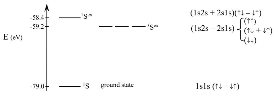
Figure 25.4.8: Several electronic energy levels of helium. There are many higher energy excited states. The first triplet state is 0.8 eV lower than the first excited singlet state.
