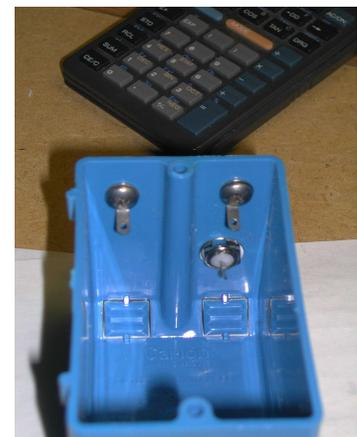
I use two screws to create binding posts on the box end that will connect to an antenna or ladder line. The choke balun shown in these instructions includes both binding posts and a coax fitting since it will be used in a variety of ways.
