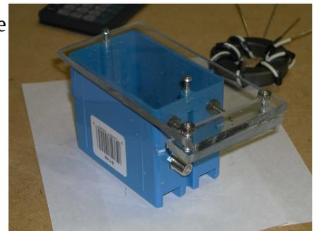
7. Placing the plastic on top of the box you can mark the two holes for screws into the box. (Shown 3 ¼ apart on the diagram.) Mark the hole with an awl. Screws will be 6-32 so holes should be drilled 5/32 inch in diameter. Mark and drill the overhang. Use the holes of the overhang to mark the clamp plastic with an awl. Drill the clamp plastic. I used ½ inch #6 sheet metal screws anchoring the top to the box.
