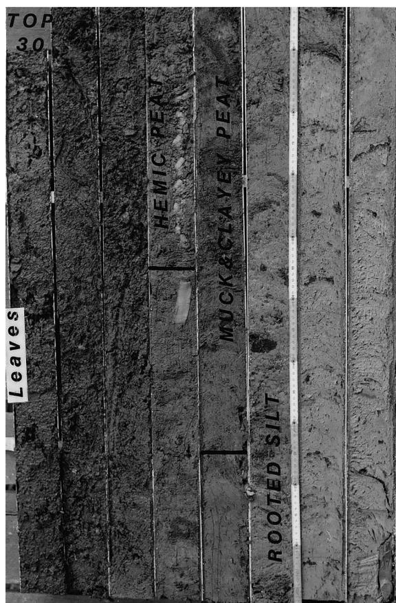
Fig. 3. Vibracore 30 illustrating the transition from poorly sorted, rooted silt to muck, clayey peat, and hemic peat. Note the position of a woody vertical root and interval from which bedded leaf litter was recovered. (Scale is in cm, with each decimeter marked on the meter stick.)
