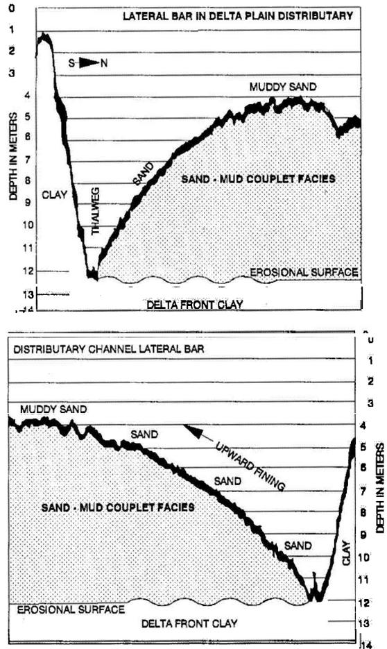
Fig. 5. Cross-sectional morphology of two distributary channels in the delta plain as reconstructed from echo soundings, surface sediment samples and vibracores.
