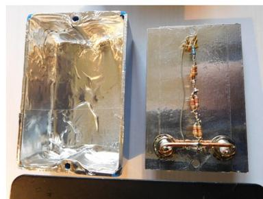
A shallow single outlet electrical box was used as a case. A cover (box lid) of clear acrylic plastic was cut to size for a cover. The through transmitter to dummy load connections are female BNC connectors. The tap for Yana is a female sma connector.
