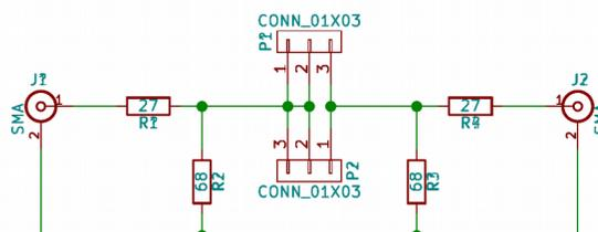
ground. Each junction (27 ohm to 68 ohm) connects to an outside pin on the pin header. The two pin headers are in parallel. The same outside pin on each header connects to the center pin on the header. The standard and unknown connect between pins 1 and 3 or 2 and 3 of P1 and P2.
