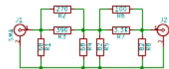
It is handy for test purposes to have a 10db attenuator. The 12.31db attenuator is close enough and easy to build, so one was made to be used for test purposes. Together the 28.64 and 12.31 db attenuators serve most test situations (in addition to calibration).
