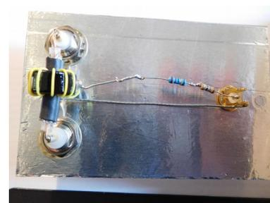
ohm resistor runs to the output to Yana. The circuit is shown at the right. RG-58 coax connects the input to the output through the core. One side of the ground braid is grounded to the coil and 10 ohm shunt.
