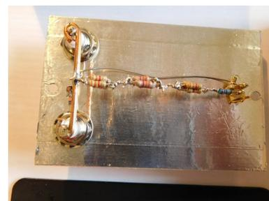
The outlet box is lined with aluminum foil duct tape with significant overlaps. The glue on the tape is not conductive, so layers must
