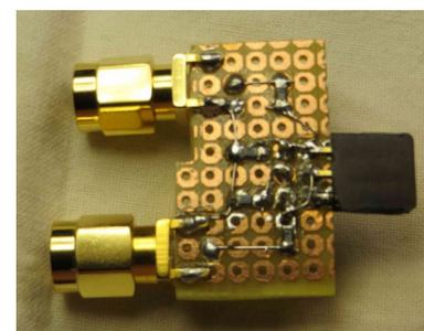
The circuit diagram shows the wiring. The photographs show my layout. A 27 ohm resistor comes off each center pin of the male sma plugs. These resistors are each connected to a 68 ohm resistor leading to
