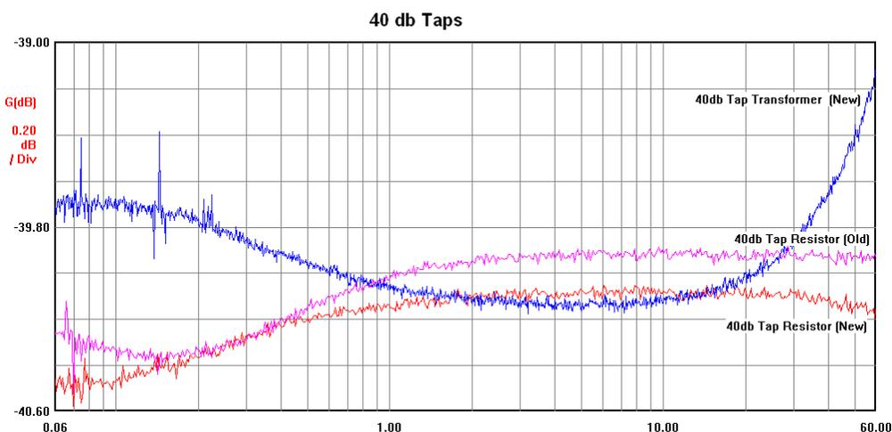
The **resistive tap** works by measuring the voltage on the coaxial line from the transmitter. The **inductive tap** measures the current in the coax. When the swr is 1:1 (as it is with a good 50 ohm dummy load) then both measuring methods give the same result for the power.
