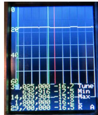
The calibration attenuator is -28.5db so that it will serve for amplifiers of gain up to 28.5db. A step attenuator would be easier to use since it could be adjusted so Yana registers 0db gain. Then the gain of the amplifier is equal to the attenuator setting.
