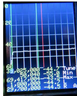
The graph at the right shows the result. Now the gain is -16db = -44.5 + 28.5. As we would expect, there is a loss between the output and the input. This figure is often expressed as  $|s_{12}|$  in db, or the **reverse gain**. It is a measure of the isolation between the input and the output.
