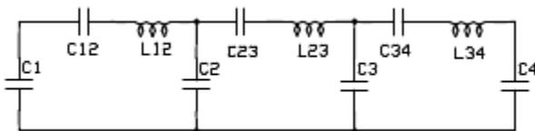
I wound the coils on FT37-61 cores with #26 enameled wire. I had to slide the turns a bit to get the right inductance. I then used coil dope (you can use clear nail polish) to fix the turns in place. Even so, the inductances are approximate (close but not equal).
