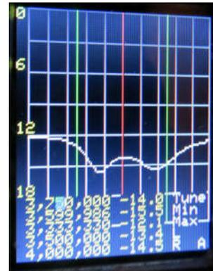
But never fear. This filter is better tuned than the "twist and check" procedure usually can achieve. Dishal's method is very robust. It worked even when I couldn't properly detune the circuits and forgot to terminate the far end of the filter in 50 ohms. Now that's a good method.
