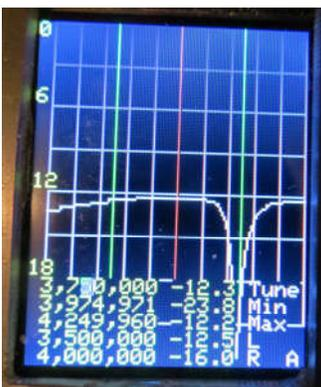
In this filter I used trimmers of fairly small value and put a fixed capacitor in parallel. Thus the adjustment is not huge. No way could I get 10 passbands of detuning. But amazingly, the Dishal method still works even with this limitation on capacitance adjustment. I think an adequate requirement is that the center tuned circuit should be at the edge or outside the edge of the passband. If this adjustment can be made, then
