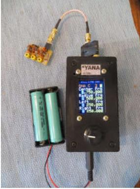
The picture at the left shows how Yana is connected to the filter through the bridge. This connection was exhibited for illustration in the experiment on filter bandwidth, but now measuring reflections will be of some use. (I forgot to terminate the “far end” with 50 ohms.)
