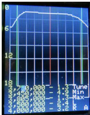
First, I tweaked the middle LC circuit tuning so that the points at which the trace crossed the green lines are at equal heights. I then used graph tuning to check the band edges.
