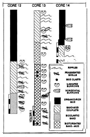
Fig. 9. Schematic representation of variability in the delta front environment between three cores recovered in close proximity to each other (Fig. 2). Organic-rich mud is characteristic of a tidal flat environment, whereas bioclastic sands characterize distributary mouth bars. For details of sediment facies see Gastaldo & Huc (1992).
