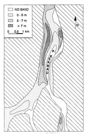
**Fig. 4.** Isopach of lateral channel bar configuration at P. Kerbau (Fig. 1). Lateral channel bars form a low sinuosity sand ribbon that consists of elliptical pods that result from the coalescence of individual lateral bars.
