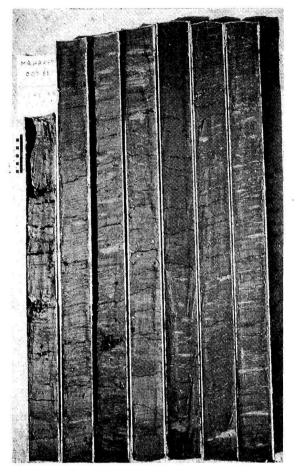
Fi.g 8. Core 33: recovered from the lateral channel bar immediately south of Tandjung Dewa (Fig. 2). Note the presence of sand and mud couplets in which thinner and thicker packages of sand-mud can be seen to alternate throughout the length of the core. Sand is concentrated in laminar, ripple and flaser-bedded structures primarily oriented downcurrent. DNAG scale is in cm.
