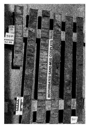
Fig. 7. Core 13: one of seven recovered from the delta front (Figs 2 & 9). Bioturbation from sand into mud is evident in the middle setion of the core. Entire and fragmentary invertebrate bioclasts are interspersed within the facies of the lowermost delta plain and delta front. DNAG scale is in cm.
