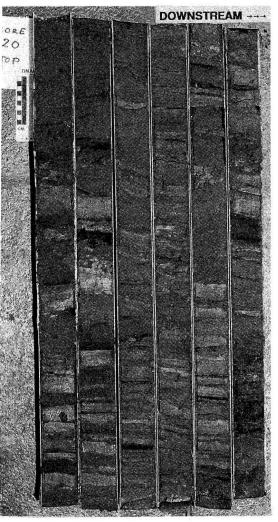
Fig. 6. Core 20: one of 10 vibracores recovered from a lateral channel bar near P. Lalukenan (Fig. 2). Note the interbedding of sand and mud, with sand disposed in isolated ripples, inclined strata and trough cross-bedded structures. Inclination of beds may be variously oriented. Core barrel is cut into 1 m sections. Top of core (sediment-water interface) is in the upper left; bottom of core is in the lower right. DNAG scale is in cm.
