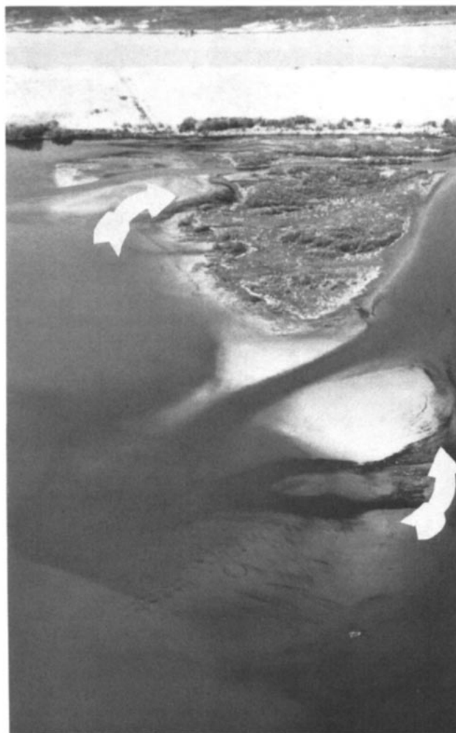
FIGURE 3 —Oblique aerial photograph of distributary mouth bar (DMB) of main crevasse channel (March, 1985). Sample was cored from approximate crest of DMB. Arrow to the right of the DMB designates the site of accumulation of macrodetritus; arrow in the upper left designates the site of the peat shoal. Sites of macrodetrital accumulations can be identified by the black tones highlighted in the shallow-water areas adjacent to the subaerial crevasse shield. Due to a change in water movement affecting the DMB of the lateral channel, the peat shoal has been covered by silty muds and slightly reworked by tidal and surficial currents.
